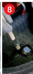
8 Seal the MINICOMBI base and any still exposed buffed areas with INNERLINER SEALER and cut the stem.
