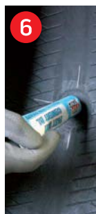
6 Apply CEMENT FD-BL on the buffed surface, fill the puncture channel with fresh cement and immediately insert the MINICOMBI plug.
