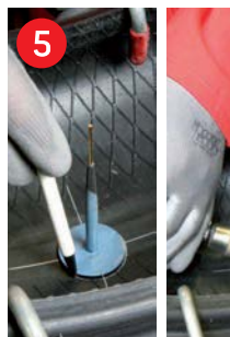
5 Buff the inner liner until you get a completely smooth surface (RMA-2) and clean the buffed area.
