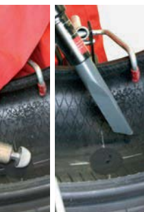
5 Buff the inner liner until you get a completely smooth surface (RMA-2) and clean the buffed area.
