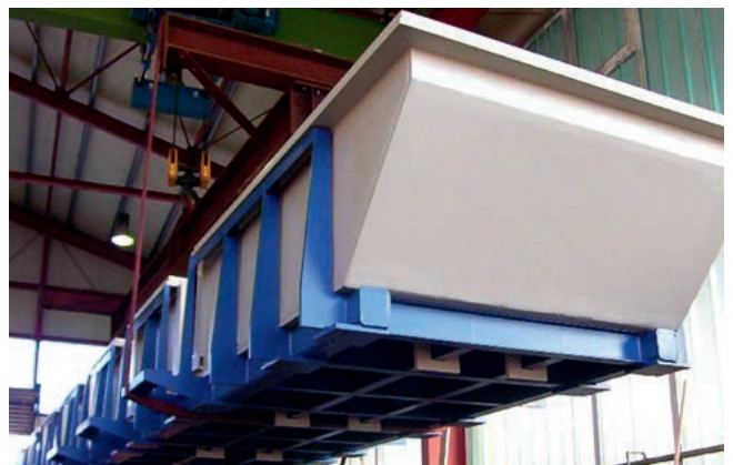
Pickling plant in PP
